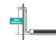
I Inner High Lift Pump
