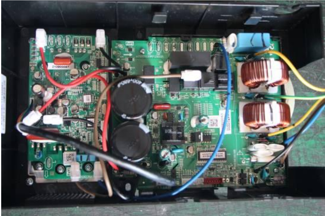
18k/24k outdoor power source board, intelligent power source board and PFC board
