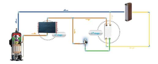
Plate Heat Exchanger as a secondary intercooler boosts up refrigerant subcooling and improves 10% energy efficiency.
