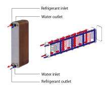
Water side heat exchanger uses multiple metal plates to achieve efficient heat transfer between refrigerant and water.
