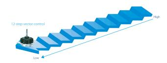
Fan speed is controlled according to the system pressure and system load, reducing power consumption by 30%.
