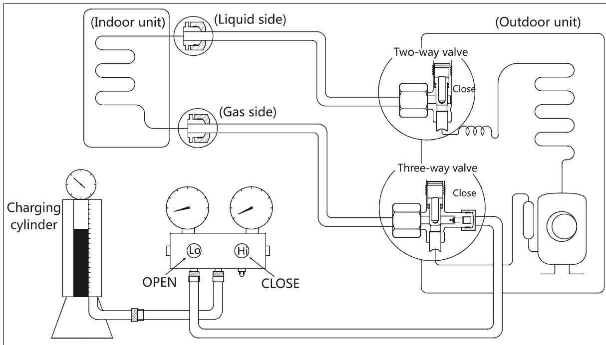
Prior to recharging the refrigerant, confirm the additional amount of refrigerant required using the following table:
